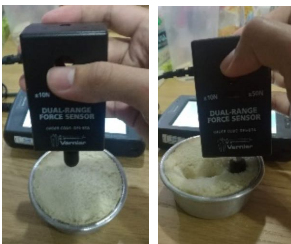
Figure 3. The Force Probe being inserted into the bread to record the force needed to puncture it using Datalogger program.
